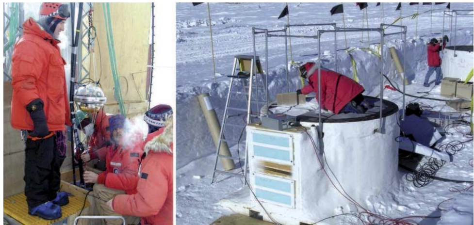
Fig. 20. – Left: deployment of an IceCube string, equipped with DOMs. Right: a tank of IceTop.
