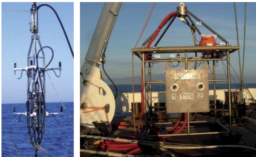
Fig. 34. – Left: an acoustic module of AMADEUS, equipped with 6 hydrophones. Right: O\nu DE before the deployment.
