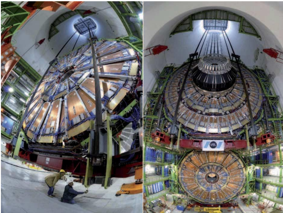
Fig. 3. – The lowering of two disks of the endcap from the surface to the underground cavern.
