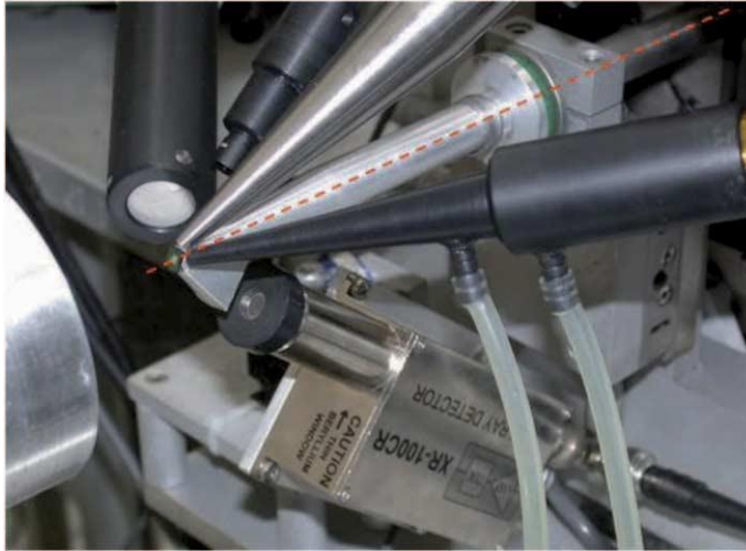
Fig. 13. – Final part of the external microbeam setup [9] at LABEC-INFN in Florence, showing in particular the system used for beam current monitoring. This includes a third X-ray detector (the one below the beamline), which detects Si X-rays from the exit window, made of an ultrathin \text{Si}_3\text{N}_4 layer. The exit nozzle is shaped with the inclined exit window and an “appendix” below (vacuum-sealed by a thin Upilex window on the rear side —not visible therefore in the picture). This exit nozzle geometry allows the dedicated detector to see only X-rays from the window; instead, those produced on the target, which is usually placed two or three mm downstream, cannot reach the dedicated detector because they are out of its unshielded sight. Also visible in the picture are the two X-ray detectors of our standard X-ray detection setup, the larger cryostat of a gamma-ray detector (on the left), a viewing camera and, above the exit nozzle, a cone containing a particle detector for backscattering measurements.
